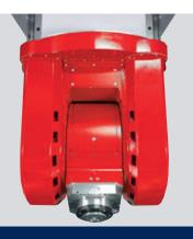
Dust and fumes can be easily conveyed by Mecof suction system integrated in the fork type milling head.
